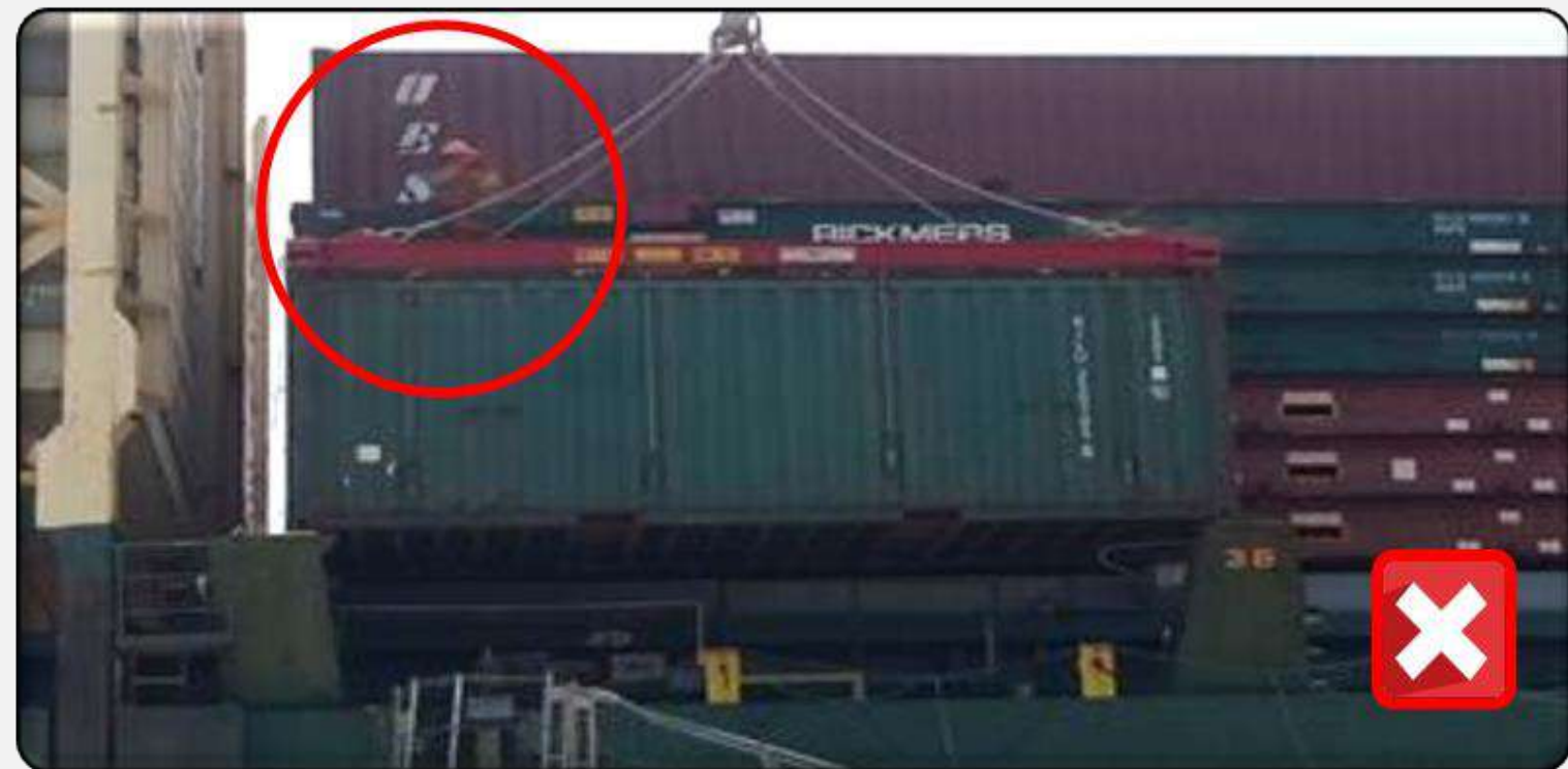
Working on top of container without fall protection
