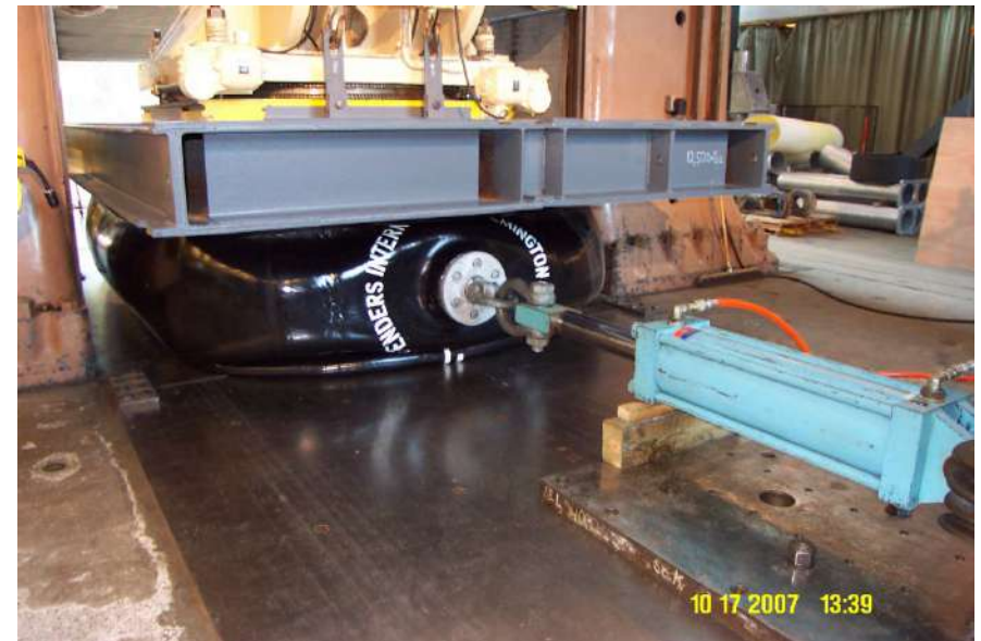
FENDER TEST AT 60% COMPRESSION
